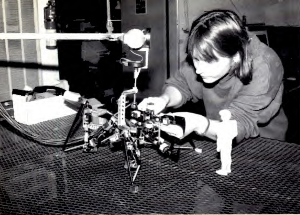
Employing skills developed in stop-motion, a "motion animator" controls the movements of a warrior bug making an adjustment on the real-time Digital Input Device, the 1996 Technical Oscar-winning invention of the Tippett Studio.
